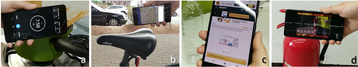
Fig. 4. Object-specific applications: knocking on (a) a pot to launch a cooking timer, (b) bicycle to mark the parking location, (c) a water bottle to order online, and (d) a fire extinguisher to view the usage instructions.
